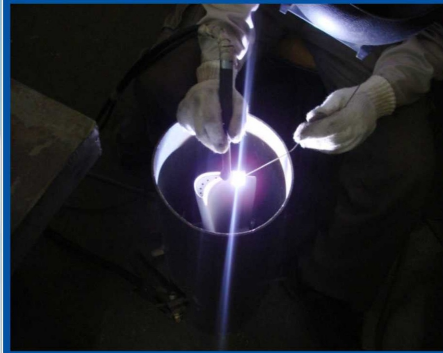
• Welding on First Stage Bucket MS 9001E using WRAP process
